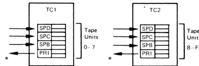
**TAPE SUBSYSTEM CABLING FOR THE DEVICE SWITCH FEATURE**
