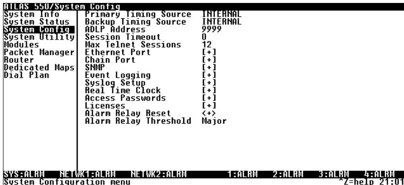
Figure 6-3. System Configuration Menu
